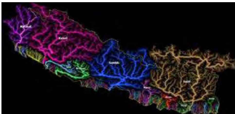
Figure 2. River networks map of Nepal derived from SRTM90m DEM (each color representing a river basin)
