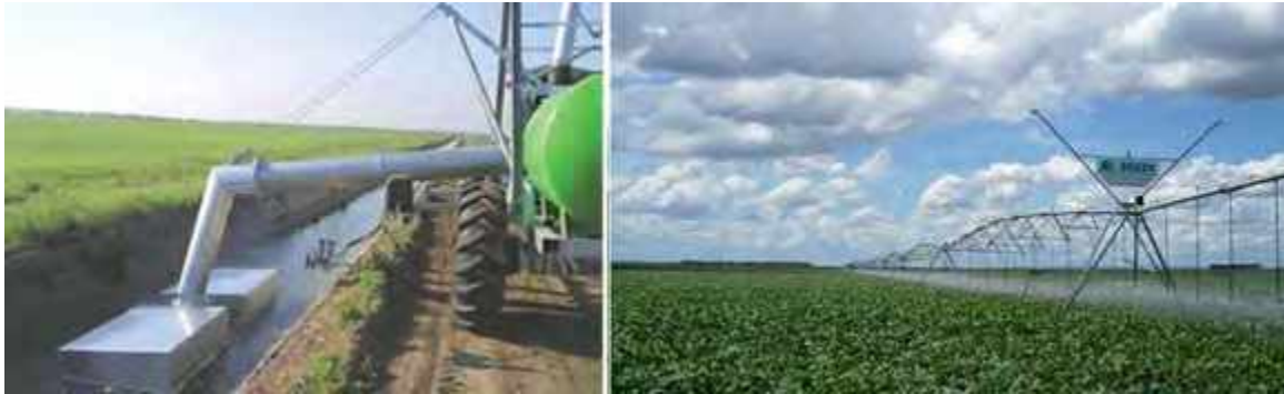
Figure 4. Water intake from the canal at the Linestar installation, sprinkling of fields with the Centerliner installation (with a circular type of movement) of the company "Bauer GmbH "(Austria).
