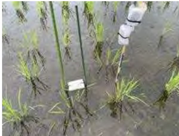
Figure 3. Temperature loggers installed in the experimental paddy plot for temperature measurement of ponded water and soil.
