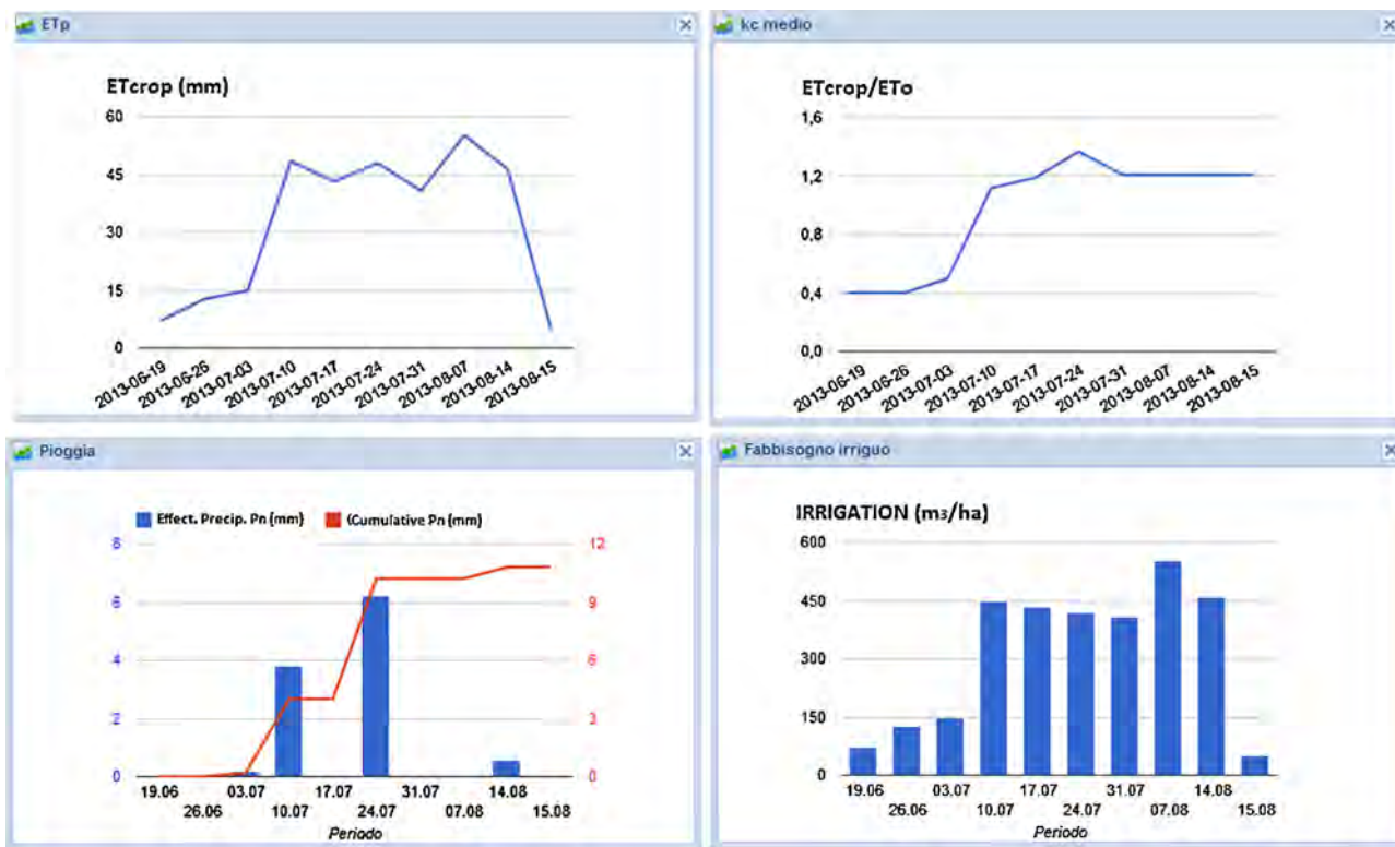
Fig. 8. Graphs of the temporal evolution of average values of ETp, effective precipitation and crop water requirements for a selected plot.
